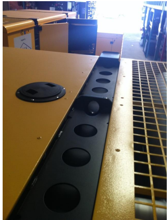
Top Crane Lift Points
